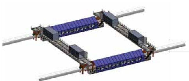
Specially designed access unit for suspension bridge maintenance. (R&D, Ålsrode Smede og Maskingfabrik & Davai Design)
