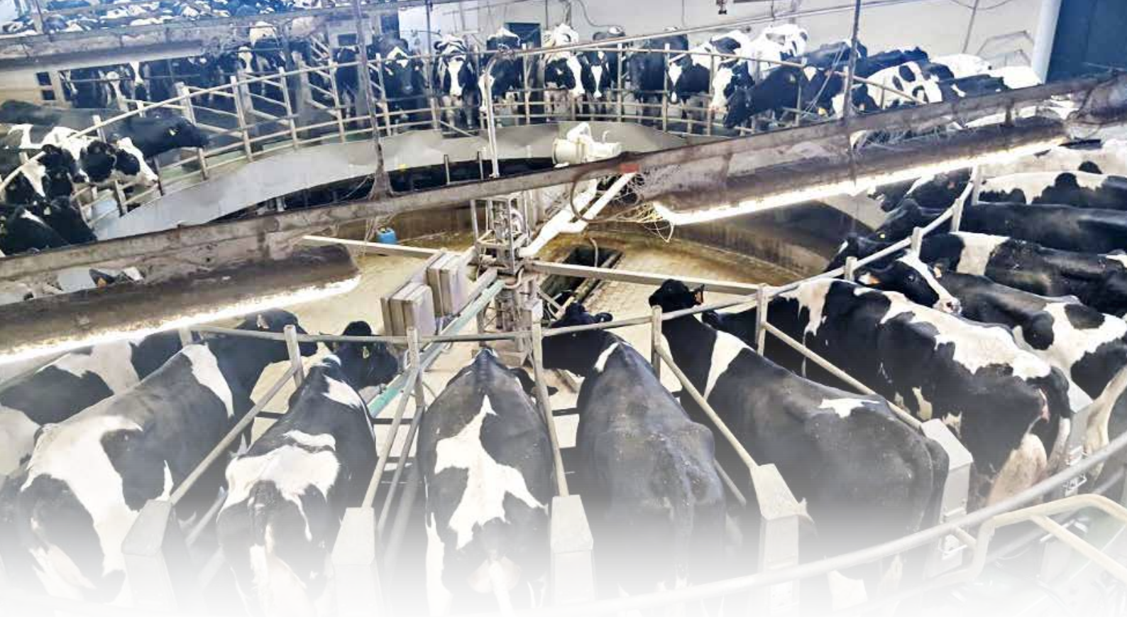
500 cows are milked twice a day in this 40-places rotary milking parlour.
