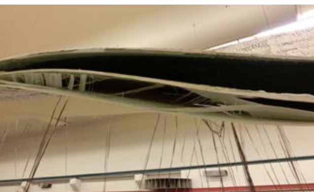
Failure of trailing edge in full-scale blade test
