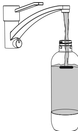
*Important! Never carbonate anything other than pure drinking water, as sugar or other additives might cause the pressure relief valves to stick, rendering the machine unsafe to use.*
