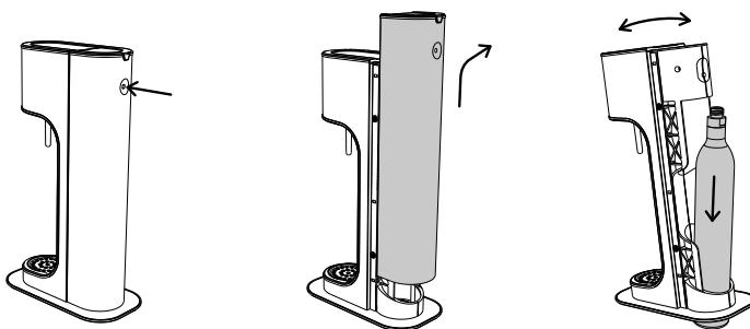
Tilt the sparkling water maker forwards and insert the gas cylinder through the opening in the bottom of the machine so that the cylinder is standing on the work surface. Gently tilt the sparkling water maker back so that the upper part of the machine rests against the threaded neck of the cylinder.
